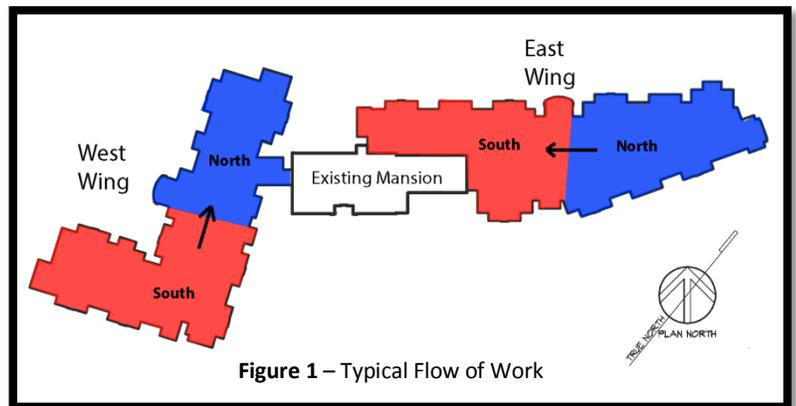
The East Wing follows the similar sequence but rather than starting on the south end, the north end was the starting point. The sequencing was phased to have the two new additions be erected toward the existing Mansion. Each wing averages about 60 days to complete the substructure and only 25 days for the superstructure to be complete.
